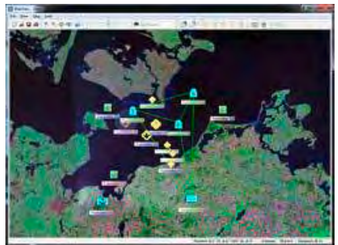
COMINT situation picture with automatically detected radio networks. The picture shows identified and unidentified radio sites marked with different tactical symbols.
