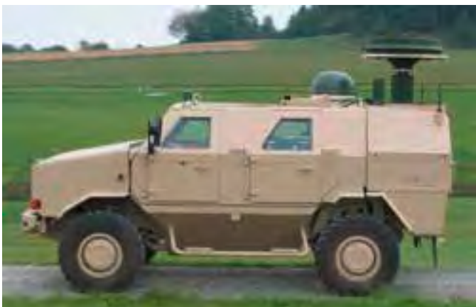
Mobile CESM system integrated into an armored vehicle.
