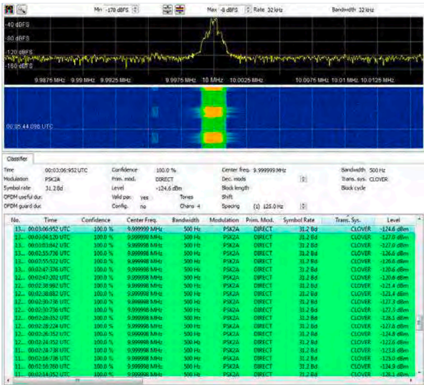
The classifier continuously measures technical signal parameters such as center frequency, bandwidth, symbol rate, modulation type and transmission system. It recognizes this signal as an HF CLOVER modem with the corresponding parameters.
