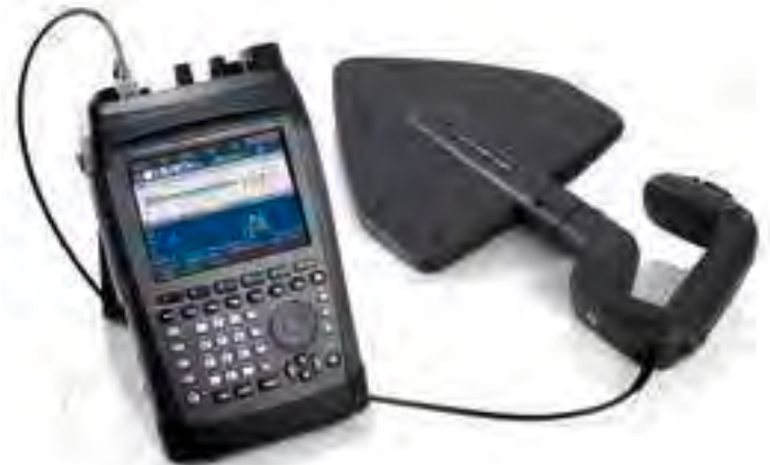
The R&S®PR100 with the R&S®HE300 active directional antenna: The antenna comes with three modules that cover the frequency range from 20 MHz to 7.5 GHz (can be expanded to 9 kHz with optional HF module). The preamplifier is accommodated in the grip piece.
