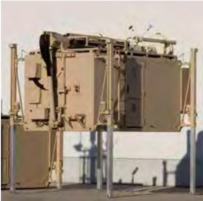
Shelter housing a semi-mobile R&S®RAMON radiomonitoring station with the mast folded down for transport on a truck.
