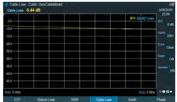
One-port cable loss measurement.
