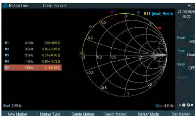
Return loss measurement – Smith chart display.
