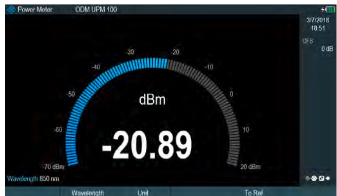
Optical power measurement with optical power sensor.
