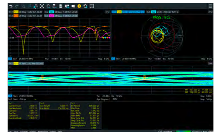
Simultaneous display of eye diagrams and measurements in the frequency and time domain.
