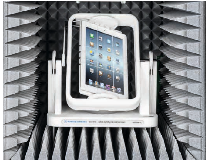
Automated 3D tablet positioner (R&S®DST-B165).
