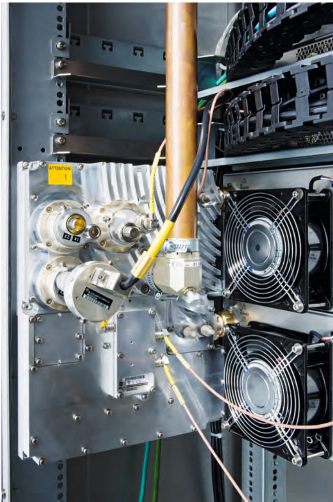
6-in-1 coupler unit for coupling two R&S®PMU901 amplifiers.
