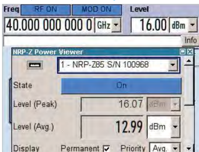
Details of the measurement with the R&S®NRP-Z85 wideband power sensor (peak and average).
