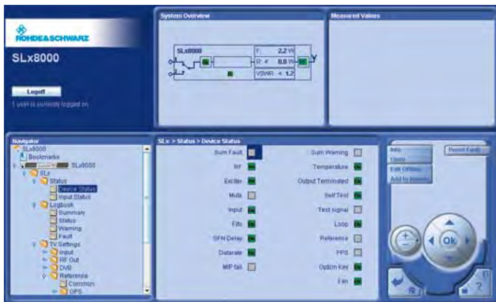
Convenient operation of the R&S®SLx8000 family of UHF/VHF transmitters via a web browser.
