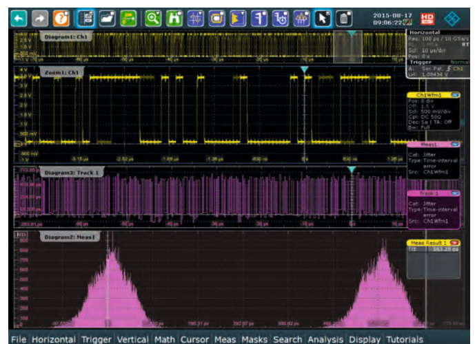
Measurement of the time interval error (TIE) of the embedded clock for different bit sequences (010000X10000001). The lower histogram shows that the TIE differs based on the bit sequence.
