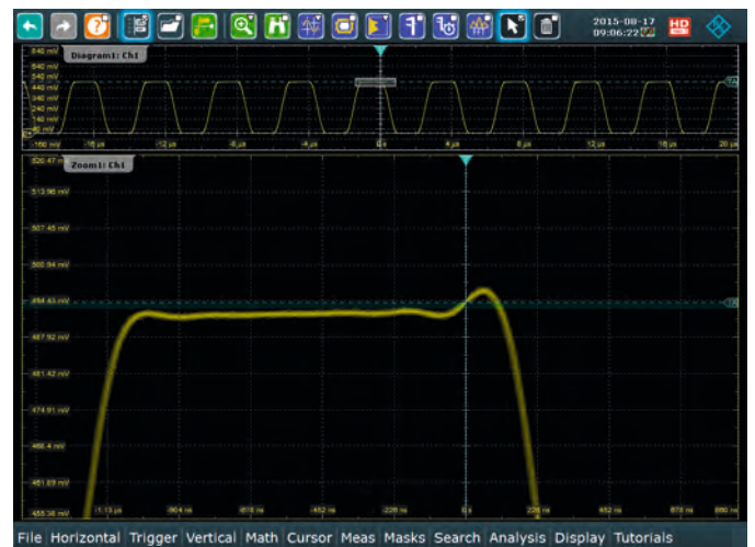
The unique architecture of the digital trigger permits stable triggering, even on signal details such as this 0.4% overshoot (high definition option).
