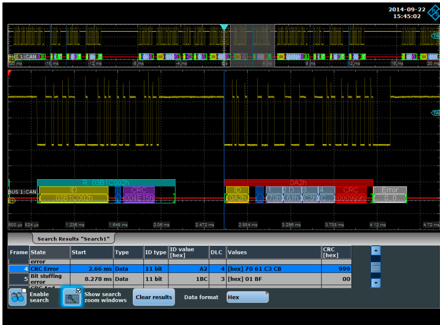
Identifying errors within a serial protocol with the R&S®RTE search function. All events are summarized in a table for easy navigation between different events. Selected events can be zoomed for detailed analysis.
