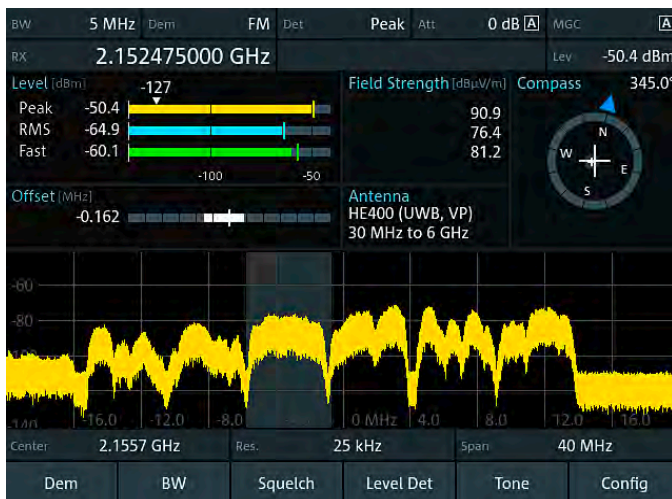
The results of up to three level detectors along with their field strength measurements can be displayed simultaneously.
