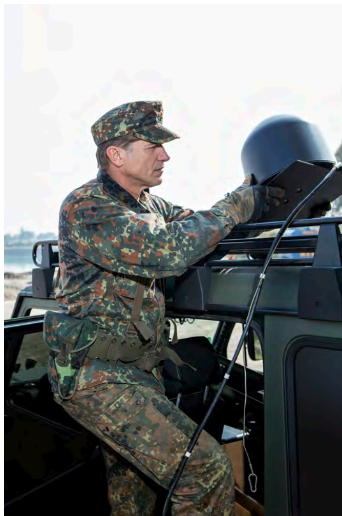
Automatic direction finding with compact DF antenna on a magnet mount (requires R&S®CS-DF option)
