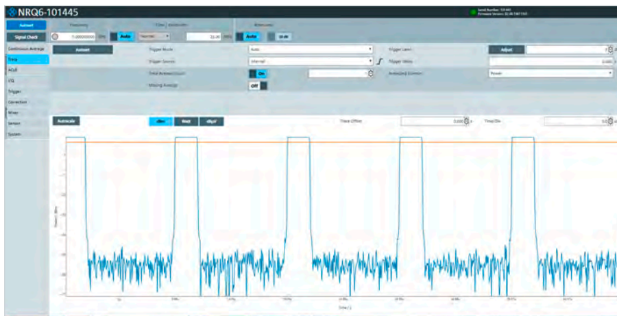
Trace measurement on a pulsed signal
