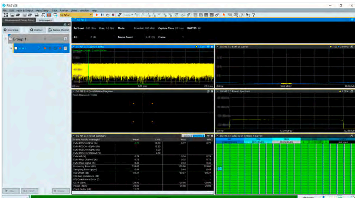
5G NR measurement with R&S®NRQ6 and R&S®VSE
