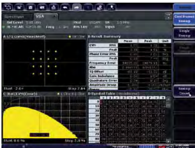
General vector signal analysis for determining the modulation quality of digitally modulated signals (16QAM).
