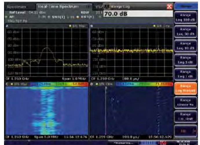
The waterfall diagram (bottom right) of the time domain display (top right) shows the pulse-to-pulse jitter of an airport radar signal. The first pulse that activates the trigger is displayed as a vertical line so that the variation in the interval to the next pulse can be clearly identified. The spectrum and the spectrogram in the frequency domain are shown on the left.
