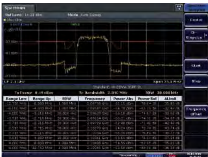
SEM measurement of a signal from a 3GPP base station.
