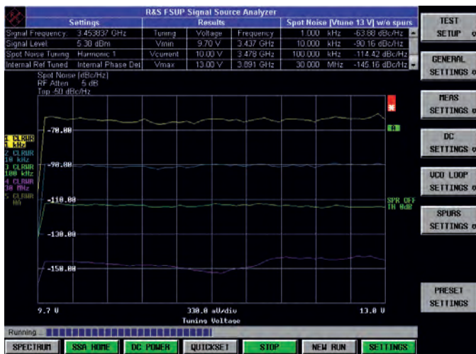
Phase noise values of an oscillator at different offset frequencies as a function of tuning voltage.
