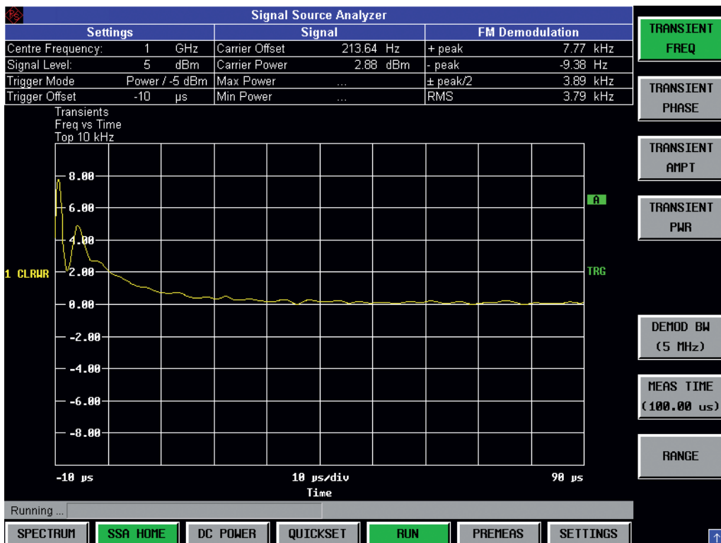
Transient response of a generator.
