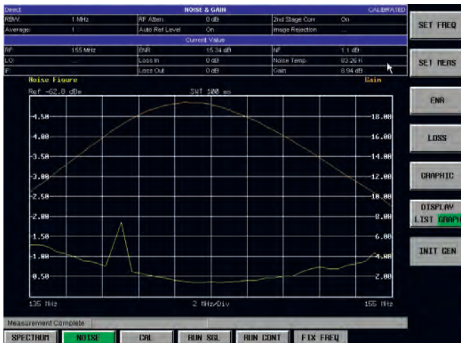
Noise figure measurement with the R&S®FS-K30 option.
