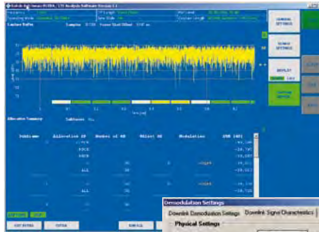
The upper part shows the power of the signal using different colors to identify important parts of the signal, e.g. the P-SCH. The lower part shows a summary of the resource blocks and their modulation quality.
