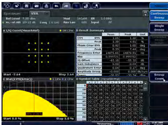
16QAM with four screens
