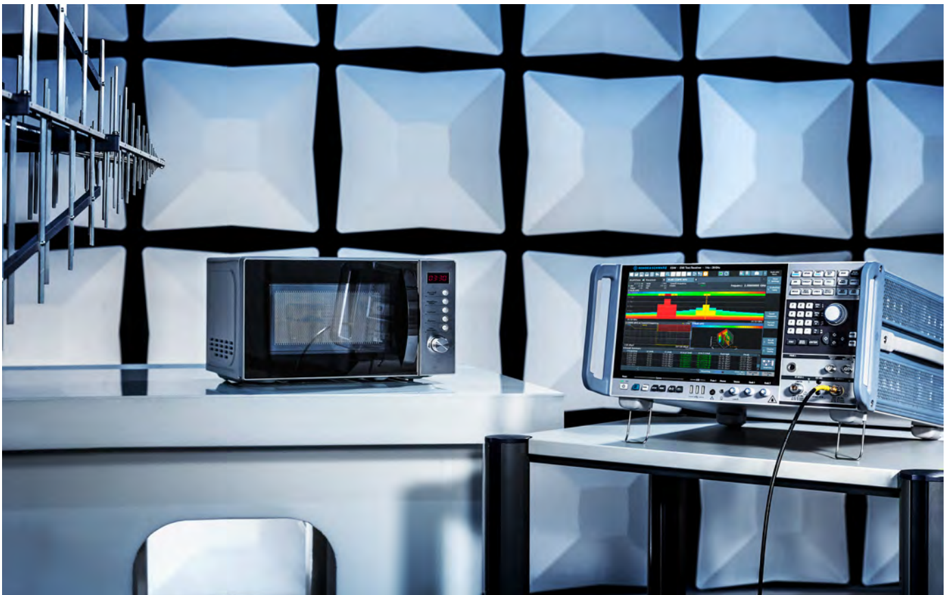
EMI testing of a microwave oven in an anechoic chamber in line with CISPR 11.
