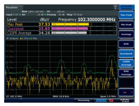
Upper part of screen: Combined numeric and bargraph level display for the current receive frequency with up to four different weighting detectors.
