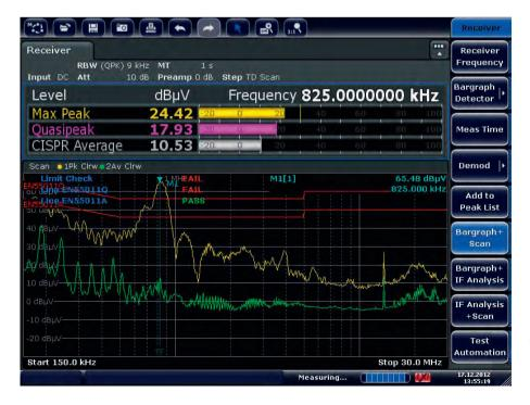
The R&S<sup>®</sup>ESRP performs disturbance voltage measurements with quasi-peak and average weighting in a matter of seconds.
