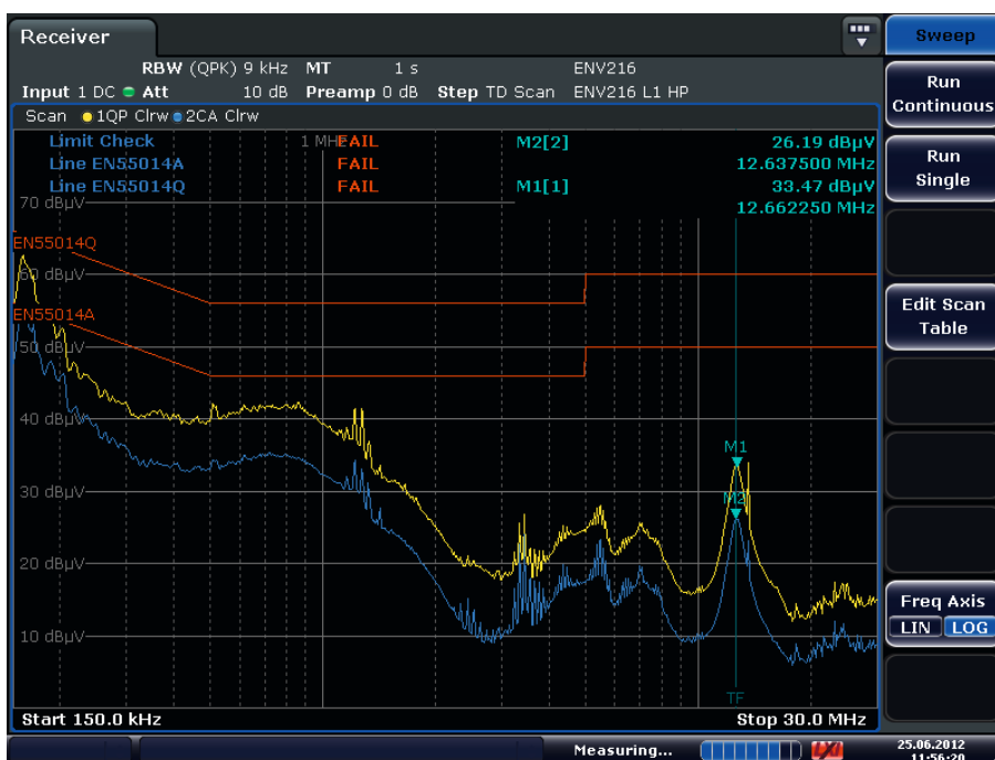
The R&S®ESR performs disturbance voltage measurements with quasi-peak and average weighting in just a few seconds.
