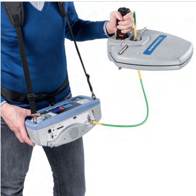
Leakage detection with the R&S®EFL110/210 and the R&S®EFL-Z100.
