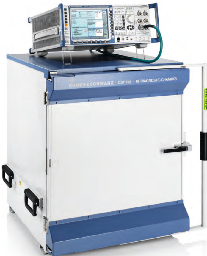
Test setup for desense measurements with the R&S®CMW500 wideband radio communication tester.
