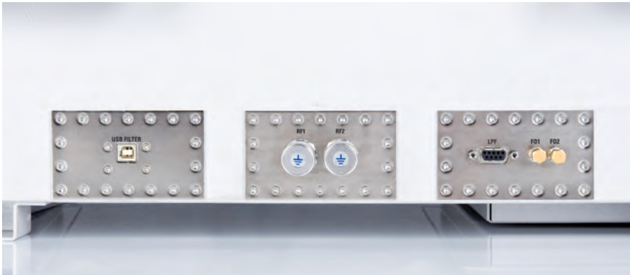
Bottom compartment containing RF and signal feedthrough connectors for conducted testing and path loss calibration.
