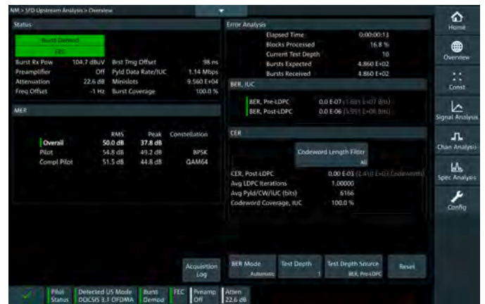
SFD upstream analysis with status display for auxiliary carrier
