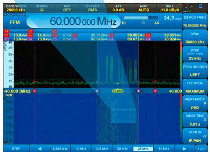
Measurement of zero span hopper timing interval
