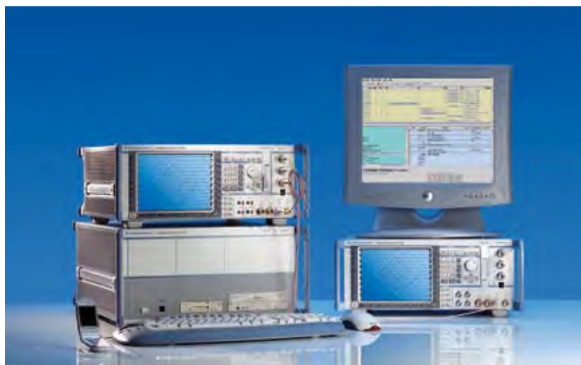
Test solution for 2G/3G intersystem handover
