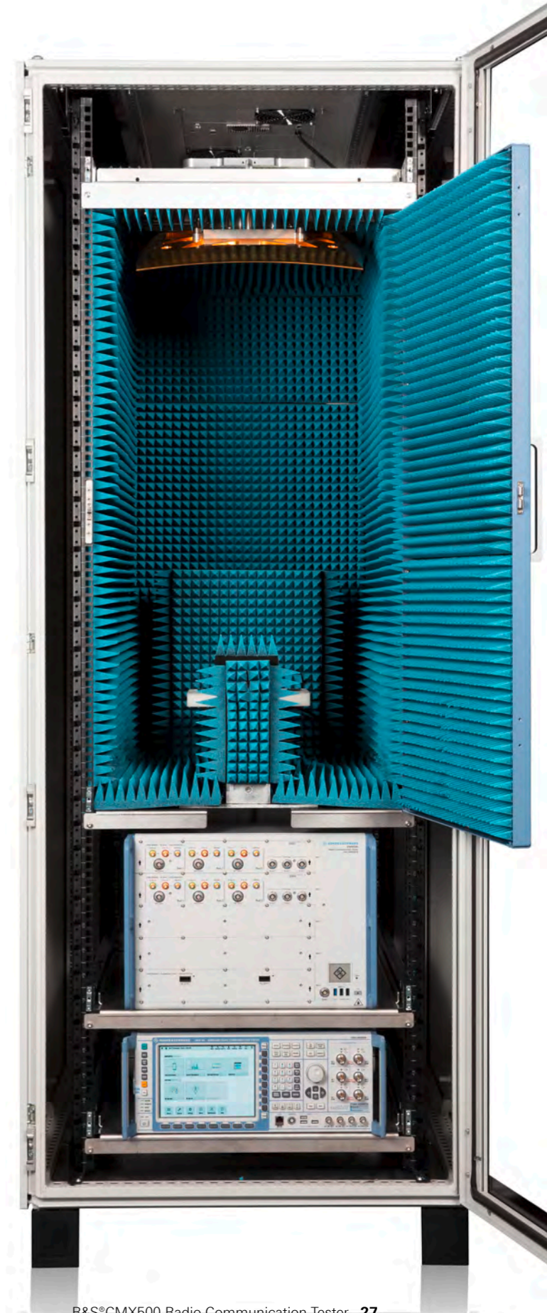
The R&S®ATS800R rack based CATR antenna test system together with the R&S®CMX500, R&S®CMW500, 2 x R&S®CMXHEAD30 and R&S®CMX-RF42 is used for the OTA setup.
