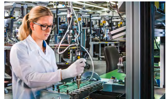
Manual component placement at the Memmingen plant, Germany.
