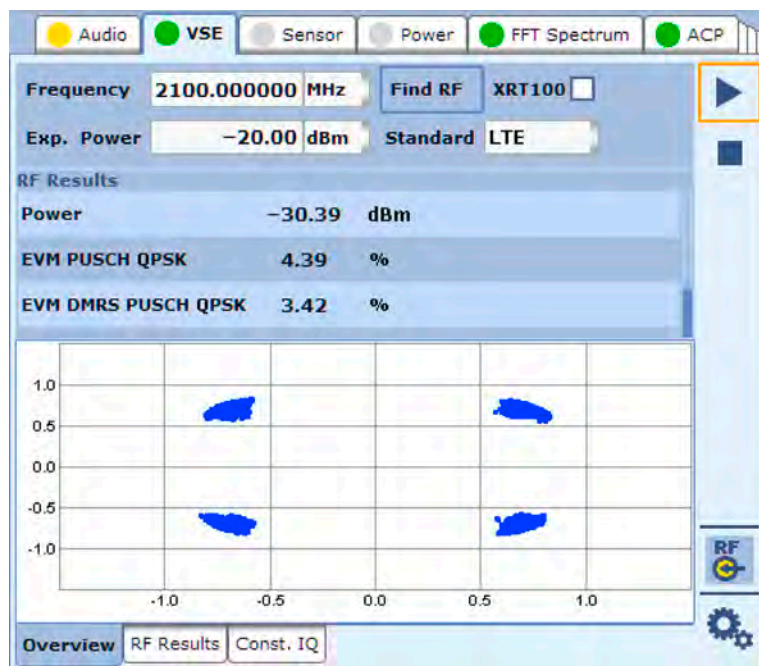
LTE transmitter measurement.
